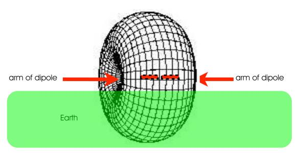
The dipole is centered in the hole of the torus pattern
