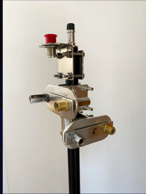
Portable Antenna with Dual Dual (Quad) Hamsticks with VHF/UHF Mount on Top - Mounted on a Photo Stand
