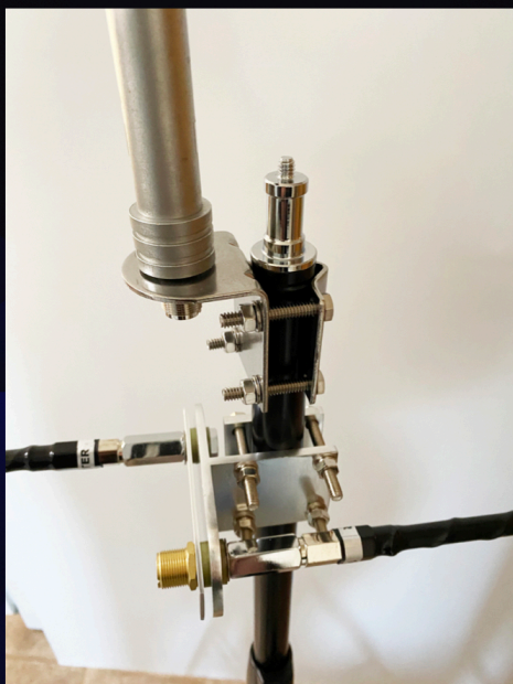
Portable Antenna with Dual Hamsticks and UHF Mount on Top - Mounted on a Photo Stand
