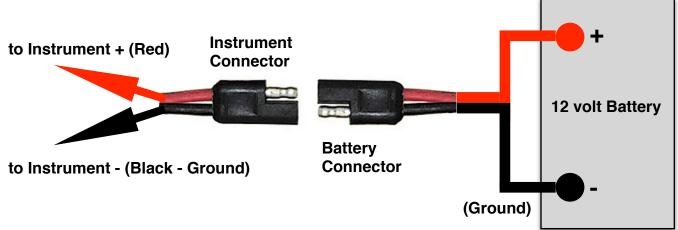
Note: instrument connector has the positive terminal exposed.
